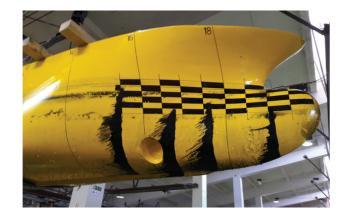
The propulsion tests were carried out in order to determine the required power at the draught of T=6.90 meters even keel and the design speed of V=15 knots. Minimum brake powers, Pbmin, of the form required for draught of T=6.90 meters is Pbmin=3490 kW at 15 knots of speed, excluding engine and sea margins.
